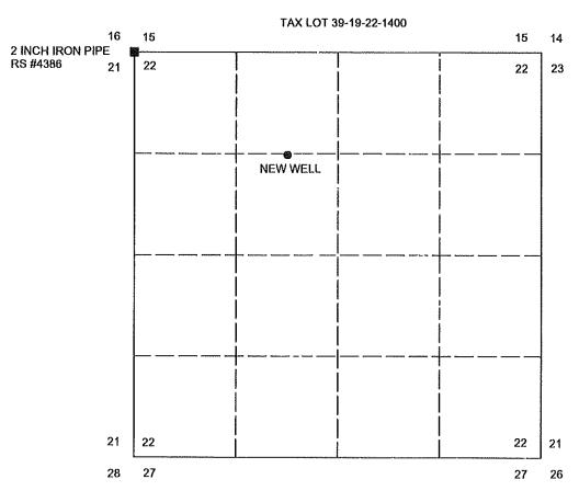
NEW WELL LOCATED IN THE SE1/4NW1/4 OF SECTION 22 AND LOCATED 1997 FEET EAST AND 1327 FEET SOUTH FROM THE NW CORNER OF SECTION 22, T39S, R19E, WM, LAKE COUNTY, OREGON
