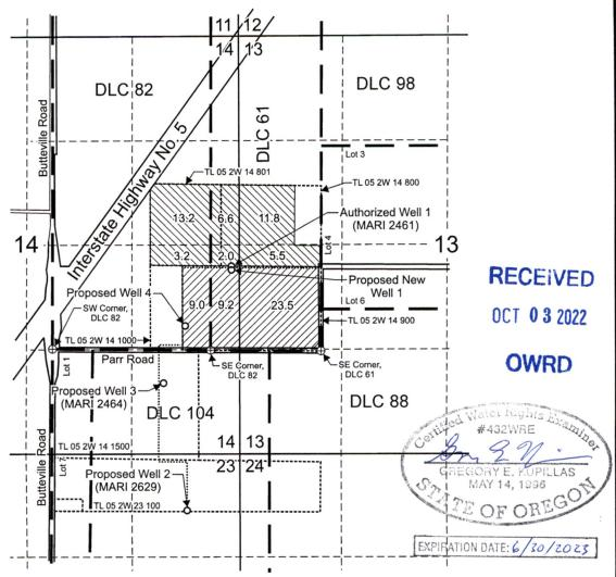
Authorized Well 1 (MARI 2461) is located 1,070 feet north and 1,130 feet west from the SE corner, DLC 61. Proposed New Well 1 is located 1,025 feet north and 1,130 feet west from the SE corner, DLC 61. Proposed Well 2 (MARI 2629) is located 2,080 feet south and 1,680 feet east from the SW corner, DLC 82. Proposed Well 3 (MARI 2464) is located 420 feet south and 1,400 feet east from the SW corner, DLC 82. Proposed Well 4 is located 310 feet north and 320 feet west from the SE corner, DLC 82.
