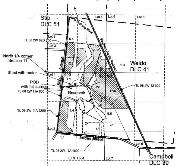
POD is located 690 feet south and 1,070 feet east from the N 1/4 corner, Section 11.
