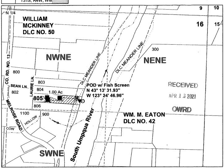
POD IS LOCATED 1151FEET SOUTH AND 1646 FEET WEST FROM THE NE CORNER, SECTION 16 AS PROJECTED IN DLC NO. 50. Legend
