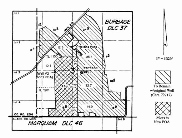
Exist'g Well is located 1930' N & 1960' E from the SW corner of DLC 37. Well #2 (add'l POA) is located 1960' N & 780' E from the SW corner of DLC 37.
