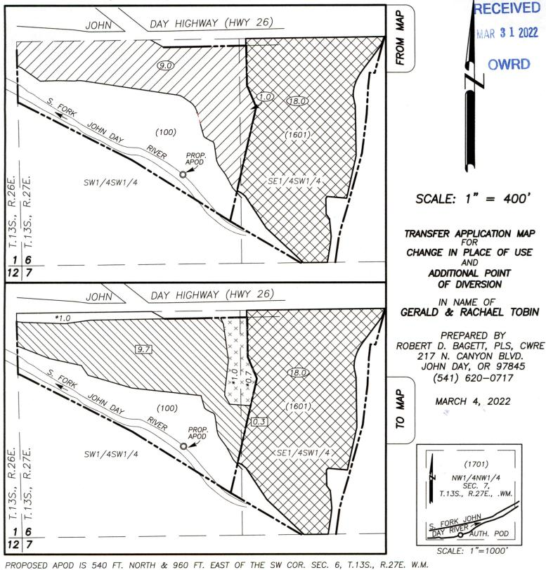
PROPOSED APOD IS 540 FT. NORTH & 960 FT. EAST OF THE SW COR. SEC. 6, T.13S., R.27E. W.M. AUTHORIZED POD IS SITUATED IN THE NW1/4NW1/4 SEC. 7, T.13S., 27E., W.M., AND IS 1240 FT. SOUTH AND 550 FT. EAST OF THE NW COR. SECTION 7, T.13S., R.27E.
