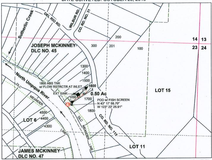
POD LOCATED 900 FEET SOUTH AND 1900 FEET WEST OF THE NE 1/4 CORNER OF SECTION 23 AS PROJECTED WITHIN DLC NO. 45. Legend
