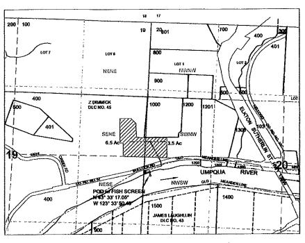
POD IS LOCATED 3000 FEET SOUTH & 80 FEET EAST OF NW CORNER OF SECTION 20 WITHIN DLC NO. 45.
