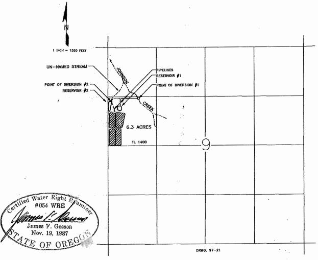
POINT OF DIVERSION #1 (FROM JOHNSON CREEK) IS LOCATED 1370 FEET SOUTH AND 840 FEET EAST; POINT OF DIVERSION #2 (FROM AN UN-NAMED SEASONAL STREAM) IS LOCATED 1450 FEET SOUTH AND 100 FEET EAST; BOTH BEING FROM THE NORTHWEST CORNER OF SECTION 9, AND BOTH BEING IN THE SW1/4 NW1/4 OF SECTION 9, TOWNSHIP 29 SOUTH, RANGE 14 WEST, W.M., COOS COUNTY.
