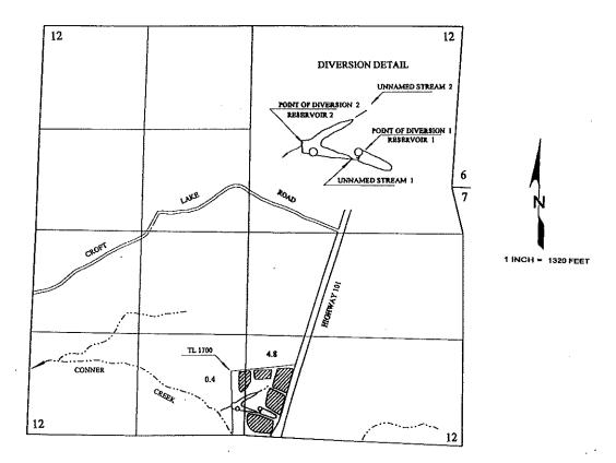
POINT OF DIVERSION No. 1 IS 310 FBET NORTH AND 200 FEET EAST WITHIN THE SW ¼ SE¼ AND POINT OF DIVERSION No. 2 IS LOCATED 330 FEET NORTH AND 80 FEET WEST WITHIN THE SE¼SW¼; BOTH FROM THE SOUTH QUARTER CORNER OF SECTION 12; WITHIN SECTION 12, TOWNSHIP 30 SOUTH, RANGE 15 WEST, W.M.; COOS COUNTY.
