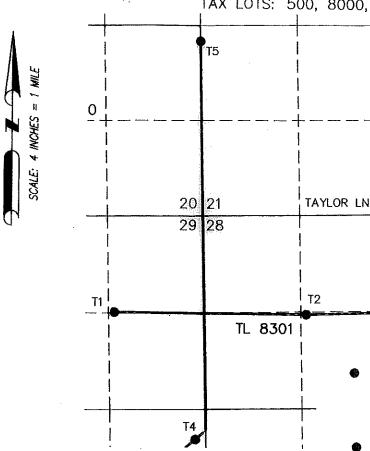
*T5 (HARN 50789)* LOCATED 2258 FEET NORTH AND 2609 FEET EAST FROM THE S 1/4 CORNER OF SECTION 20, T24S R32.5E, W.M. FLOWMETER IS LOCATED 4.5 FEET WEST FROM WELL.
