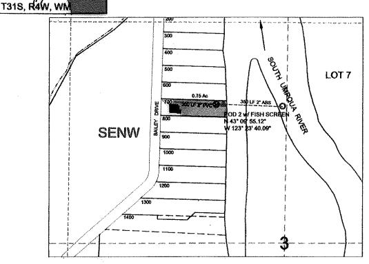
POD IS LOCATED 800 FEET NORTH & 80 FEET WEST OF C1/4 CORNER OF SECTION 3.
