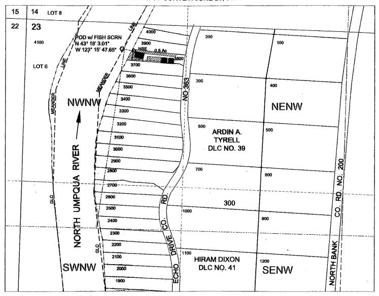
POD IS LOCATED 197 FEET SOUTH & 833 FEET EAST OF NW1/4 CORNER OF SECTION 23 AS PROJECTED WITHIN DLC NO. 39.
