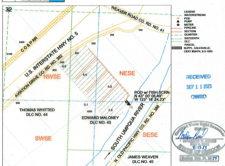
POD IS LOCATED 1285 FEET SOUTH AND 1885 FEET EAST FROM C1/4 CORNER, SECTION 32 WITHIN DLC NO. 43.
