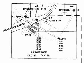
DIVERSION I - 92 - 10 IS LOCATED 680 FEET SOUTH AND 260 FEET EAST FROM THE NORTHWEST CORNER OF SECTION 19, BEING WITHIN SECTION 19, TOWNSHIP 27 SOUTH, RANGE 5 WEST, W.M.; AND DIVERSION I - 92 - 24 #I IS LOCATED 1030 SOUTH AND 330 WEST FROM THE NORTHEAST CORNER OF SECTION 24, BEING WITHIN SECTION 24. TOWNSHIP 27 SOUTH, RANGE 6 WEST, W.M.
