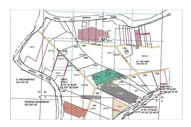
CERT 51968 POD1 IS LOCATED 620 FEET NORTH & 20 FEET WEST FROM SE CORNER, SECTION 32 AS PROJECTED IN LOT 1. CERT 90972 POD2 IS LOCATED 2300 FEET SOUTH & 850 FEET EAST FROM W1/4 CORNER, SECTION 32 AS PROJECT IN LOT 9. TRANSFER TO POD IS LOCATED 100 FEET SOUTH & 850 FEET WEST FROM THE NE1/4 CORNER, SECTION 5 AS PROJECTED IN LOT 6.
