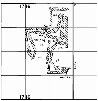
WELLS LOC: #1-2050'S. \$1560'W. #2-3780'S. \$360'W. } ALL FROM N. 1/4 COR. SEC. 16. Pump Loc: 1500'S. \$1480'W.
