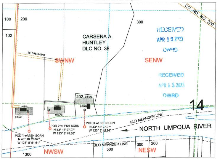
POD1 IS LOCATED 381 FEET SOUTH & 274 FEET EAST OF W1/4 CORNER OF SECTION 14 AS PROJECTED WITHIN DLC NO. 38.
