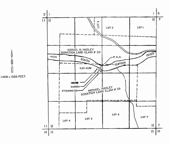
THE POINT OF DIVERSION (HANLEY SPRING) IS LOCATED 2880 FEET NORTH AND 2720 FEET WEST FROM THE SOUTHEAST CORNER OF SECTION 12, BEING WITHIN THE SE 1/4 OF THE NW 1/4 OF SECTION 12, TOWNSHIP 29 SOUTH, RANGE 6 WEST, W.M., DOUGLAS COUNTY.
