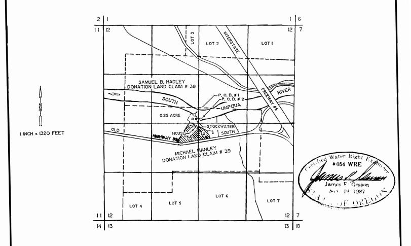
POINT OF DIVERSION #1 (HANLEY SPRING) IS LOCATED 2880 FEET NORTH AND 2720 FEET WEST FROM THE SOUTHEAST CORNER OF SECTION 12, BEING WITHIN THE SE 1/4 OF THE NW 1/4 OF SECTION 12. POINT OF DIVERSION #2 (SOUTH UMPQUA RIVER) IS LOCATED 2760 FEET NORTH AND 2540 FEET WEST FROM THE SOUTHEAST CORNER OF SECTION 12, BEING WITHIN THE SW 1/4 OF THE NE 1/4 OF SECTION 12, BOTH POINTS OF DIVERSION BEING WITHIN TOWNSHIP 29 SOUTH, RANGE 6 WEST, W.M., DOUGLAS COUNTY.
