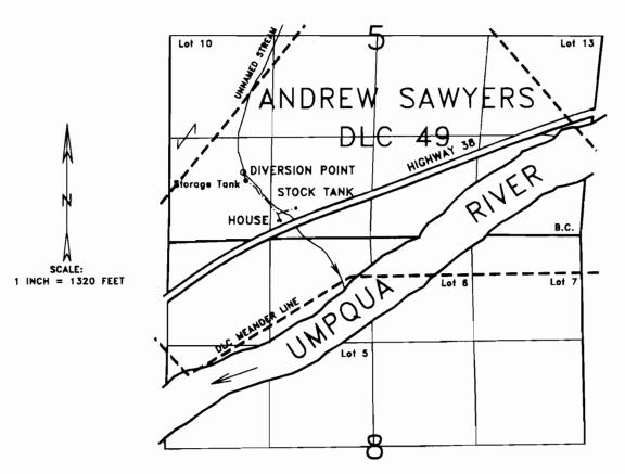
THE DIVERSION POINT IS LOCATED 800 FEET NORTH AND 4300 FEET WEST FROM THE SOUTHEAST CORNER OF SECTION 5.
