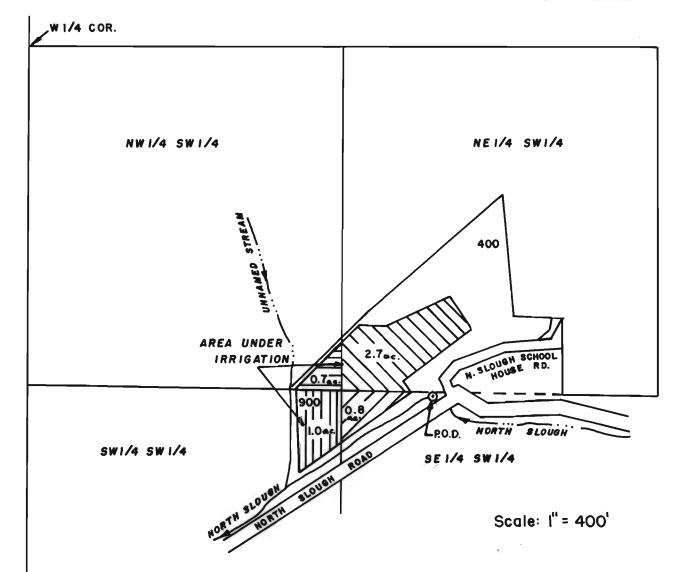
The point of diversion is \$50°06'E, 2220' from the W1/4 corner between sections 11 & 12.
