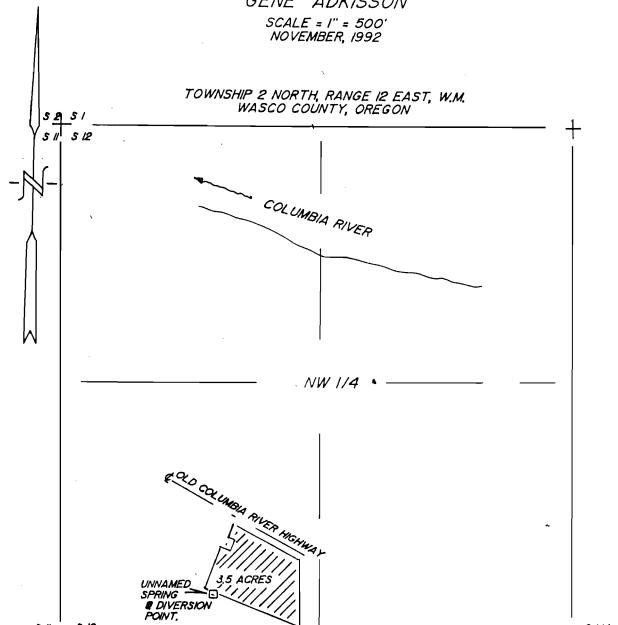
THE DIVERSION POINT IS LOCATED 207 FEET NORTH & 800 FEET EAST OF THE WEST QUARTER CORNER OF SECTION 12.
