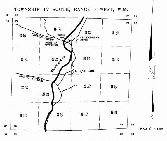
POINT OF DIVERSION: N 6 53' 24" W 1514.25' FROM THE CENTER 1/4 OF SECTION 29.
