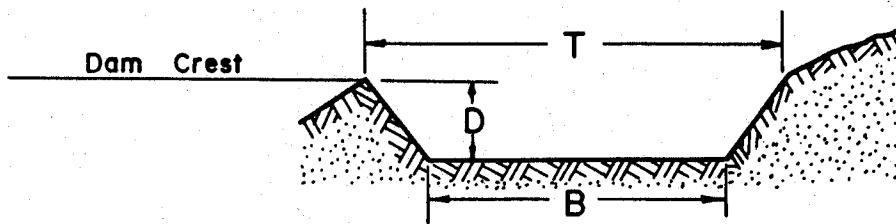
The bottom width of the spillway, B, will be ..... 8..... feet.
