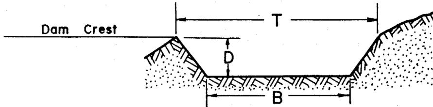
The bottom width of the spillway,  $B$ , will be 1.2 feet.
