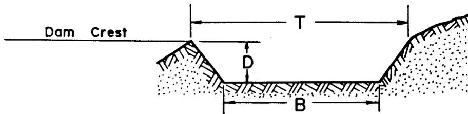
The bottom width of the spillway, B, will be 22 feet.
