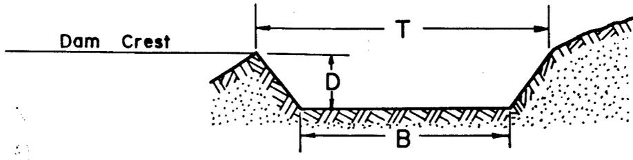
The bottom width of the spillway, B, will be 6 feet.
