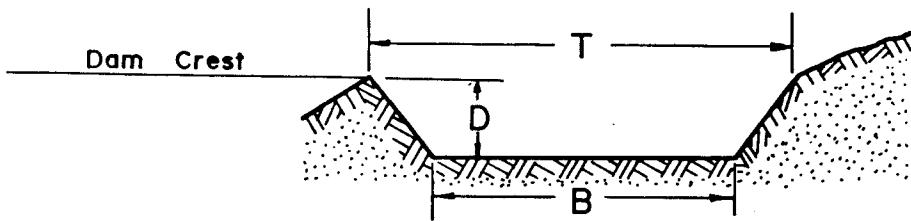
The bottom width of the spillway, B, will be ..... 10 feet.
