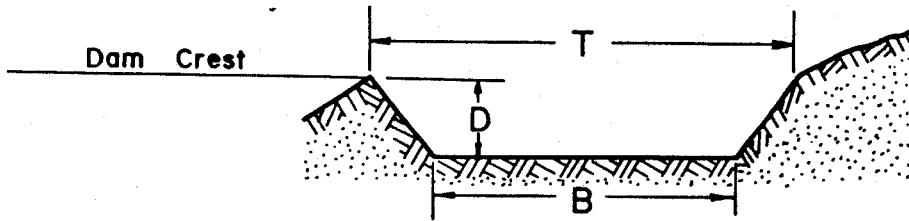
The bottom width of the spillway, B, will be ..... 5 ..... feet.
