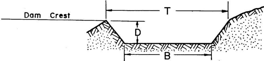
The bottom width of the spillway, B, will be 6.10 feet.
