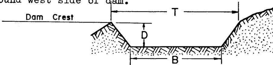
The bottom width of the spillway, B, will be all spillways 12 feet.
