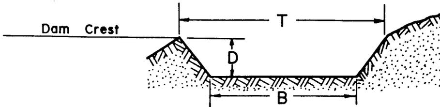
The bottom width of the spillway, B, will be 6 feet.
