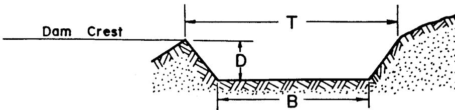
The bottom width of the spillway, B, will be ..... 50 ..... feet.
