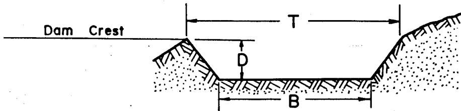
The bottom width of the spillway, B, will be ..... 100..... feet.
