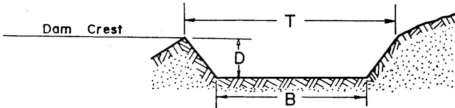
The bottom width of the spillway, B, will be .....2.4..... feet.
