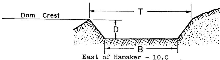
The bottom width of the spillway, B, will be .....feet.
