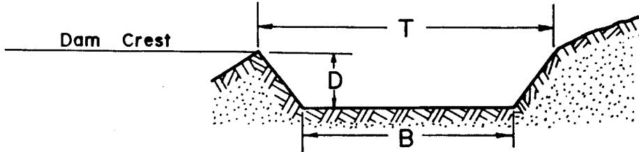
The bottom width of the spillway, B, will be ..... 8<sup>0</sup> feet.
