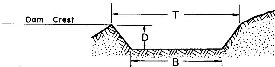
The bottom width of the spillway, B, will be .....1 1/2..... feet.
