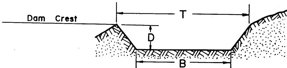
The bottom width of the spillway, B, will be 12 feet.
