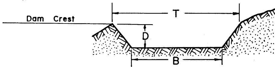
The bottom width of the spillway, B, will be 4 feet.
