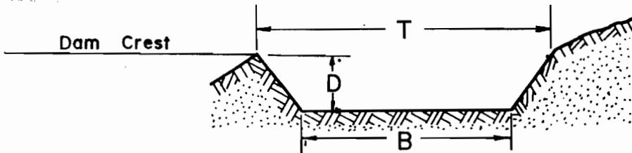
The bottom width of the spillway, B, will be 1.4 feet.
