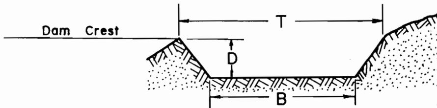
The bottom width of the spillway, B, will be 28 feet.
