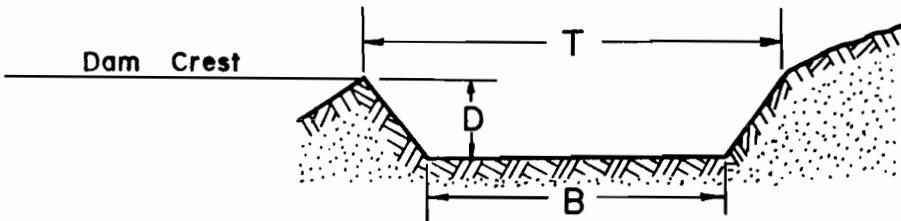
The bottom width of the spillway, B, will be .....2.0 feet.
