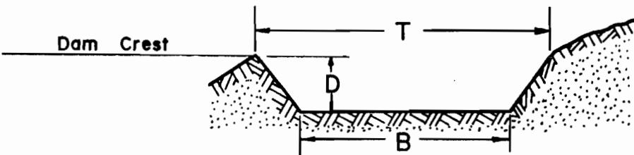
The bottom width of the spillway, B, will be ..... 2.7 feet.
