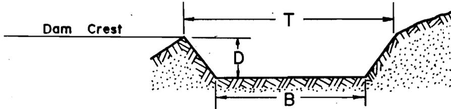
The bottom width of the spillway, *B*, will be 2 feet.
