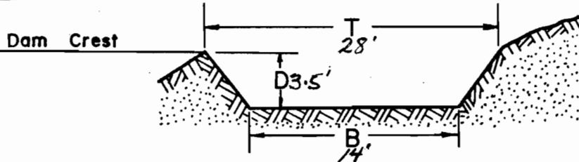
The bottom width of the spillway, B, will be ..... 14 feet.
