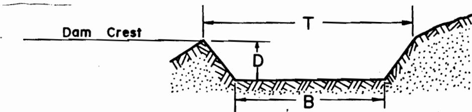
The bottom width of the spillway, B, will be ..... feet.
