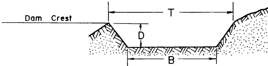
The bottom width of the spillway, B, will be ..... feet.
