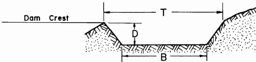
The bottom width of the spillway, B, will be ..... 15 feet.
