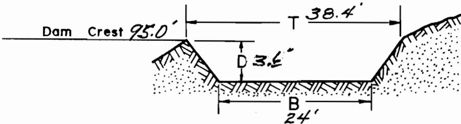
The bottom width of the spillway, B, will be ..... 24 ..... feet.
