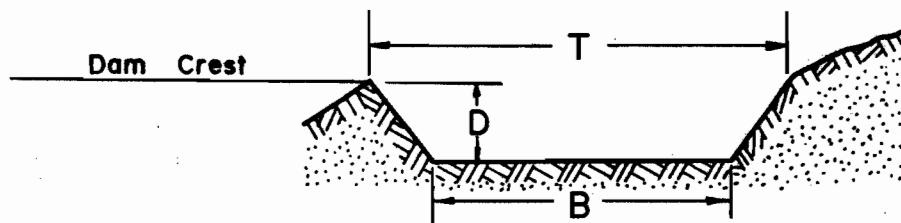
The bottom width of the spillway, B, will be..... 6.0..... feet.
